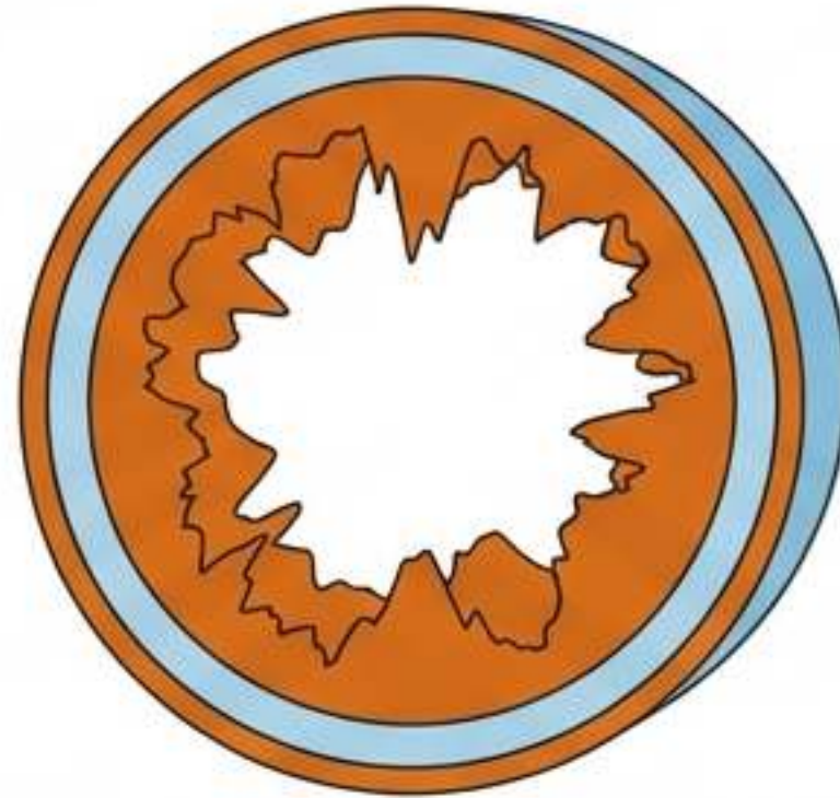
Operating State: Fouled Tube
